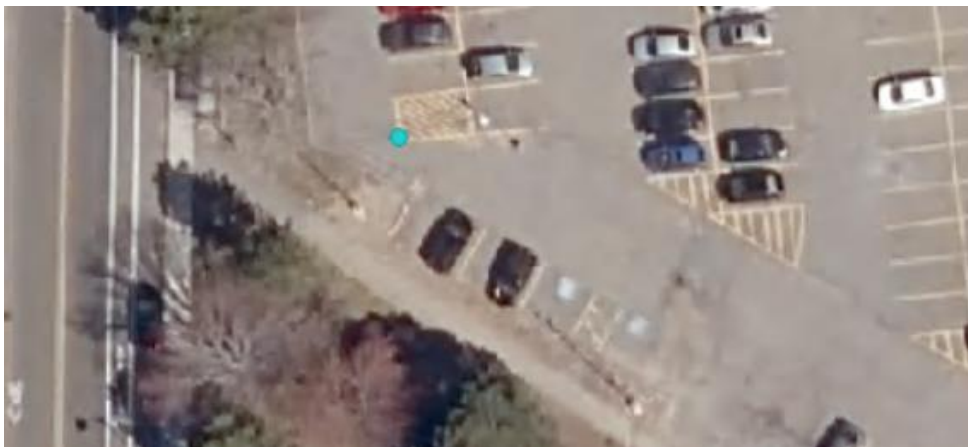
Figure 1: The permanent ground control point is colored in blue. Ground control points must be determined carefully: In this particular case, these parking indicators were scraped and repainted, so this one was not used.
