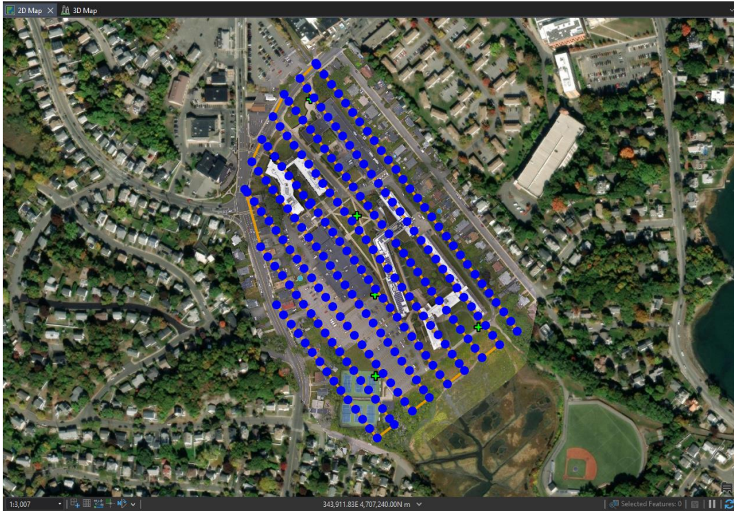
Figure 2: Each blue mark represents a photo taken, totalling at 229 photos for this flight location, Central Campus. Drone2Map is able to automatically align UAV imagery according to the placement of ground control points, shown with green crosses. (GCPs).
